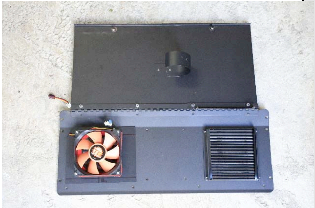
Showing black plastic fitted over the grill to block excess air pathway (fan is sucking air from unit)
